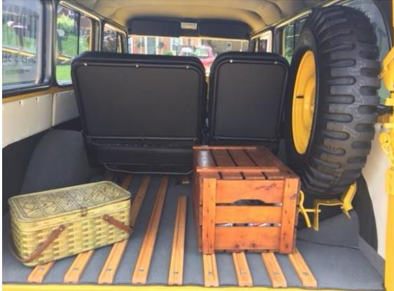
window felt strips, carpet, headliner, wind lace and new oak floor strips were installed. Everything that needed replating was sent out for straightening and chromed. Coker Firestone Military NDT tires were mounted to the original rims.
